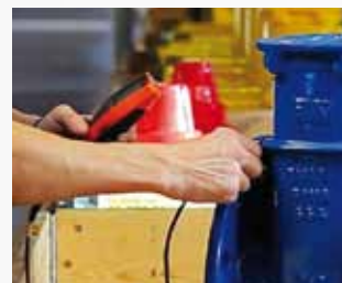
The epoxy layer thickness must be min. 250 \mu on all surfaces
