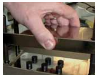
The rubber is deformed by 25 % at the compression set test
