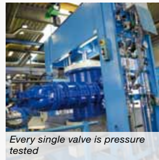
An infrared eye controls the pressure test automatically
