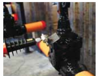
Each valve is pinhole tested
