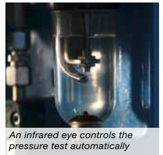
Every single valve is pressure tested
