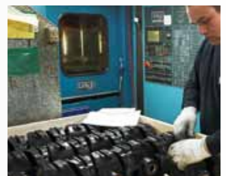
Wedges are vulcanized with min. 4 mm on all sealing surfaces
