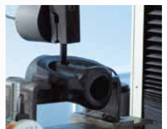
A thin layer of rubber must remain after the peeling test
