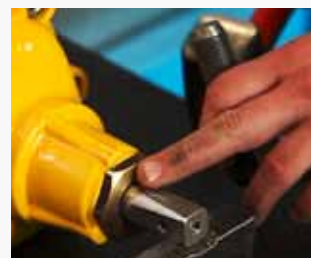
Date and serial no. are stamped on the stems of gas valves
