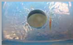
The impact resistance is tested with a steel cylinder
