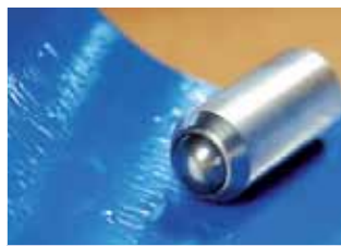
The impact resistance is tested with a steel cylinder
