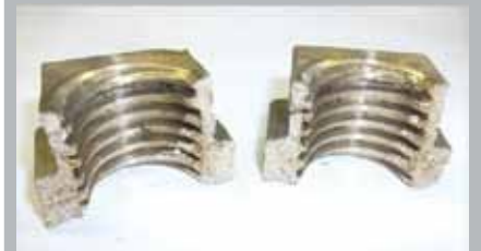
Broken wedge nut
