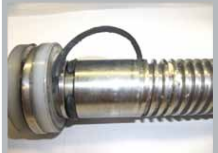
Damaged spindle thread and O-ring
