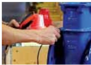
The epoxy layer thickness must be min. 250µ on all surfaces
