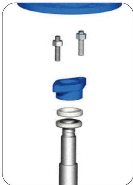
Left: Exploded view of Stem/ Packing/ Gland/ Studs and Bolts.
