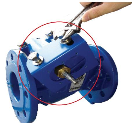
3. Mount the bracket with the new bolts and distance pieces. The longest distance piece in the upper bolt hole.
