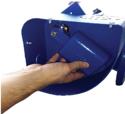
6. Make sure that there is enough play between the back plate, the lever and the weight.
