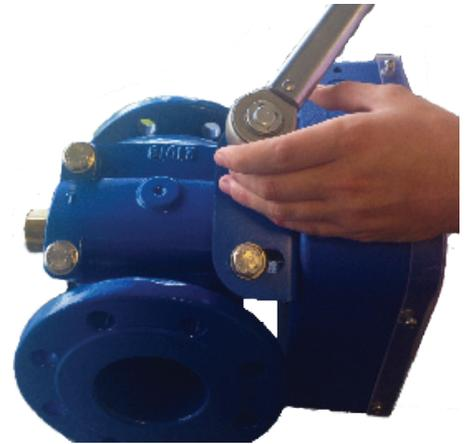
7. Tighten the bolts connecting the bonnet and body. Tighten bonnet bolts using a torque wrench set at 25Nm to 30Nm. Reset the torque wrench at 40Nm to 50Nm
