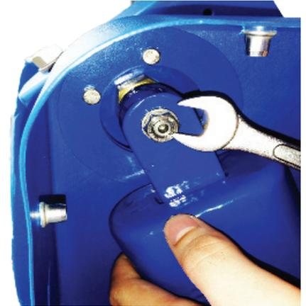
5. Mount the lever and weight on the shaft.
