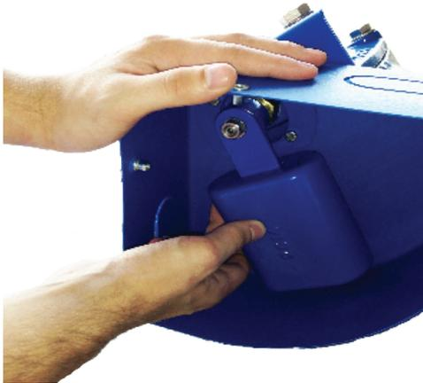
4. Adjust the back plate according to the position of the lever and weight. Screw the back plate onto the bracket. The back plate has 2 positions, a horizontal and vertical position. the back plate is positioned correctly when 4 screws can be mounted.
