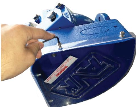
8. Mount the clear protection guard to the back plate with the screws evenly set.
