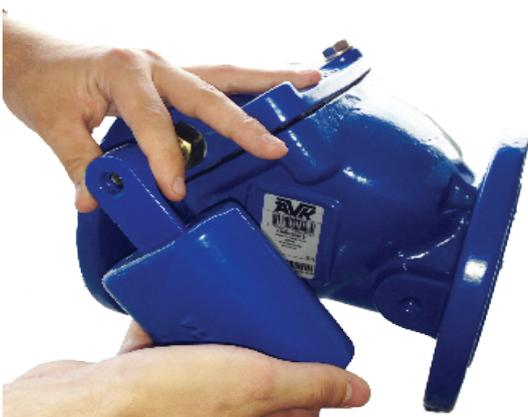
2. Loosen and remove the nut and washer on the shaft end, and remove the lever and weight.
