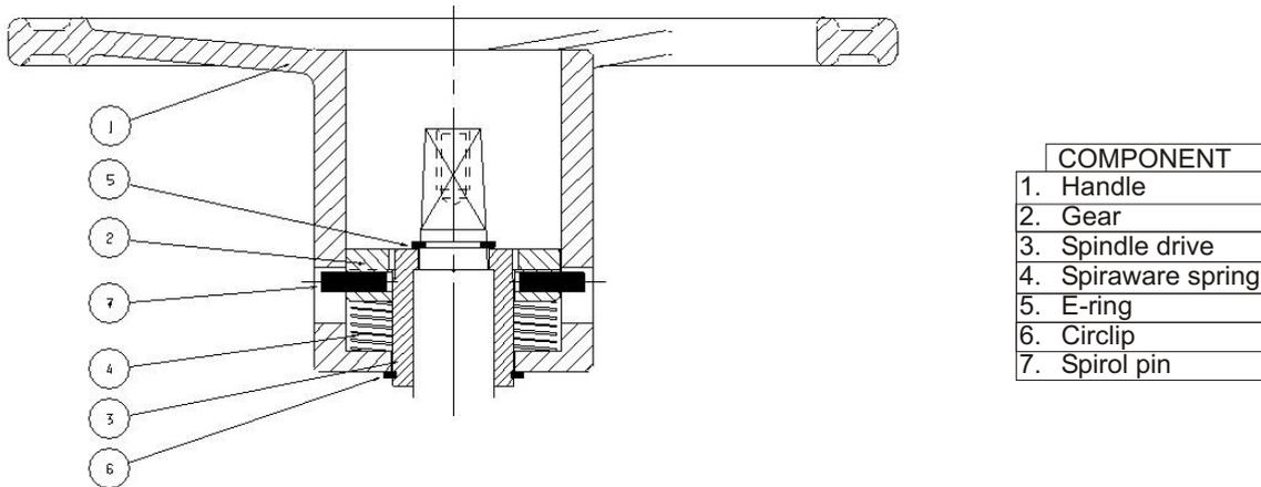
1. Remove the plastic cover fitted in the top of the Handwheel.
