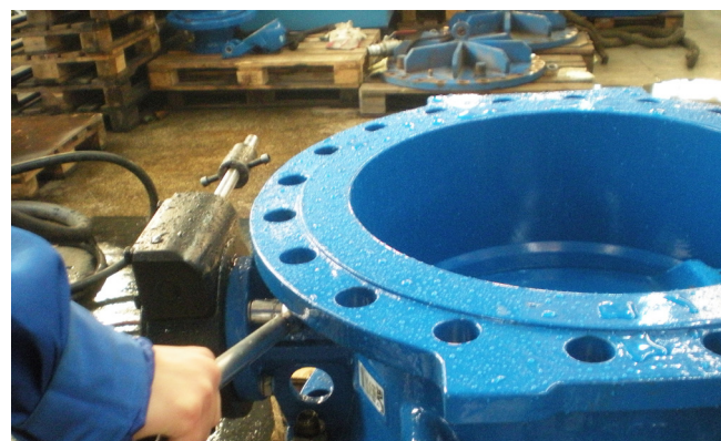
Mounting the gearbox – step 5
