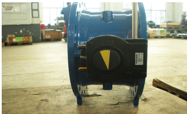
Check of position indicator – step 4
