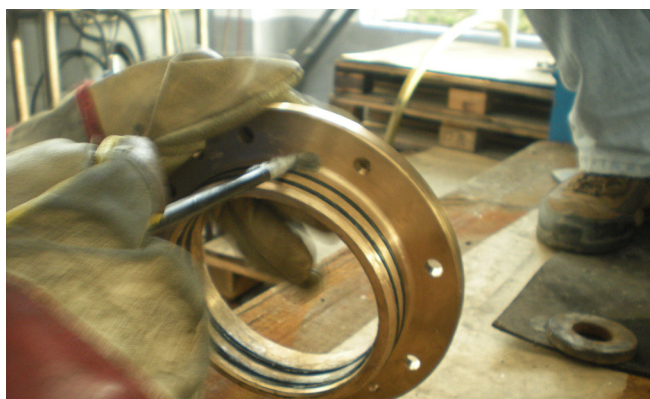
Mounting and greasing of O-rings – step 3
